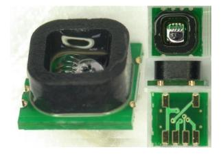
A soft gel coating provides some measure of environmental protection, none the less, it is not recommended to expose this sensor to conditions of high moisture or corrosive chemicals. The sensor is housed in a surface mount package, and uses materials that are compliant with United States of America and European Union standards on hazardous material content.
