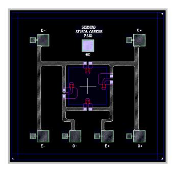
The MTPD2000 series piezo-resistive pressure sensor dies are manufactured on six inch silicon wafers in a class 100 clean room using a state of the art 1.2 micron CMOS facility and are then bulked micro-machined in a class 1000 clean room. The wafers are batch manufactured using a electrochemical etch stop process to achieve excellent repeatability.
