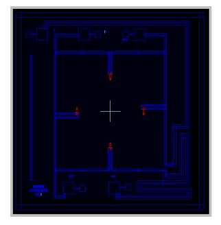
The MTPD007 series piezo-resistive pressure sensor dies are manufactured on six inch silicon wafers in a class 100 clean room using a state of the art 1.2 micron CMOS facility and are then bulked micro-machined in a class 1000 clean room. The wafers are batch manufactured using a electrochemical etch stop process to achieve excellent repeatability.
