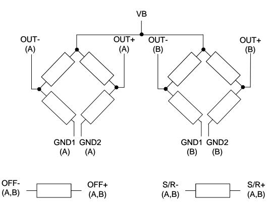
Pin Configurations (Arrow indicates direction of applied field that generates a positive output voltage after a SET pulse.)
